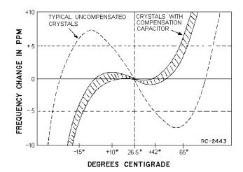
Figure 2 - Typical Crystal Characteristics
