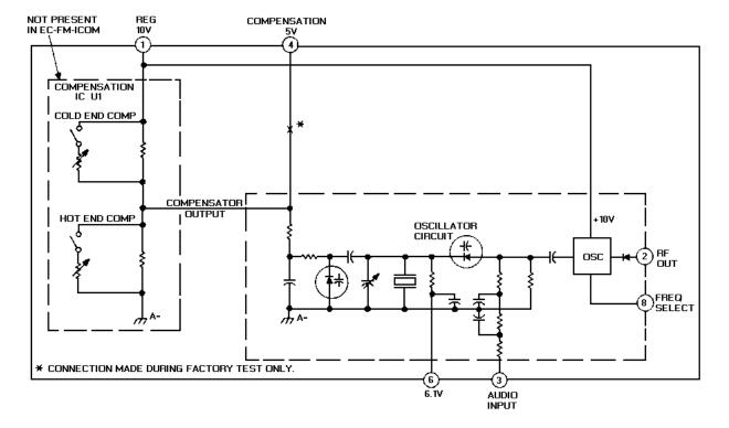
Figure 3 - Equivalent FM ICOM Circuit
